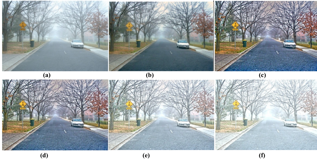
Fig. 2. Simulation Results with change of \omega value (a) Original foggy 'road' image (b) Output at \omega = 0.95 of He et al. [4] method (c) Output of proposed method at \omega = 0.95 shows oversaturated effect (d) Output of proposed method at \omega = 0.9 shows minimized oversaturation and smooth sky region (e) Output of proposed method at \omega = 0.5 and (f) at \omega = 0.2 shows no obvious visibility improvement.
